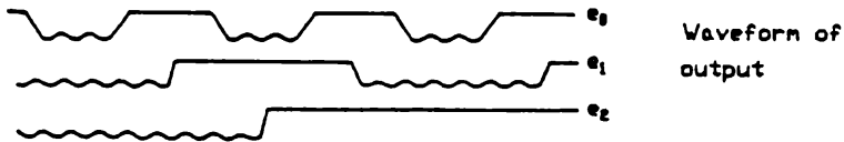
Fig. 12 Actual response of the encoder using Fig. 11 circuit.
