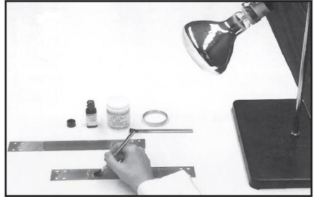
Figure 1 – PhotoStress coating being brushed on steel test specimens of different alloy content for the purpose of studying the post-yield strain behavior.
