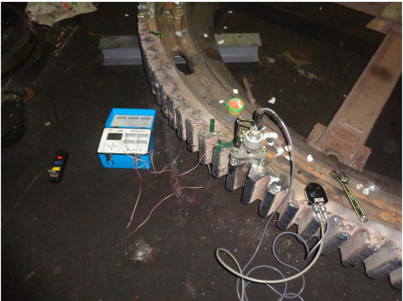
Figure 2: Evaluation of Residual Stress on workpiece using RS-200 Residual Stress Milling Guide and P3 Strain Indicator and Recorder
