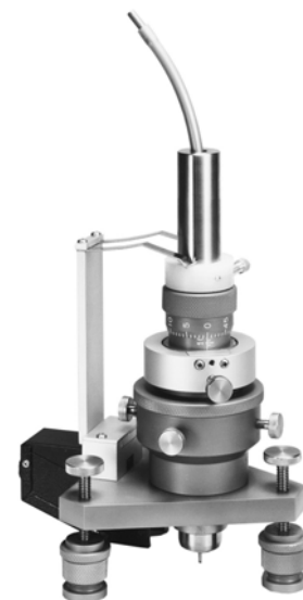
Figure 1: RS-200 Milling Guide for Residual Stress Measurements
