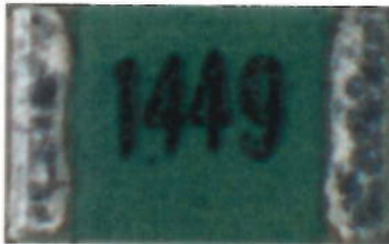
FRSM-0805 chip with INK marking Date Code (Year / week)
