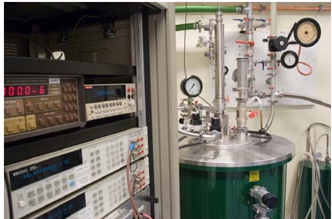
Figure 1: VSL quantum Hall resistance standard.
