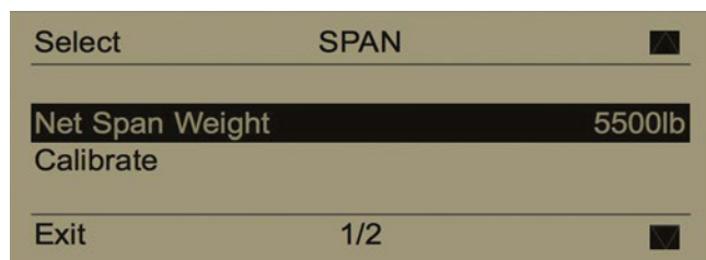
Fig 3.15 Press Select to edit the Axle Span as required.
