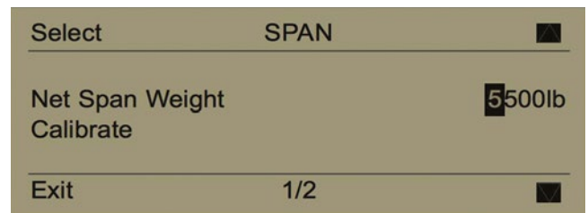
Fig 3.16 Enter the calculated span weights. Press Exit once when the weight has been set.
