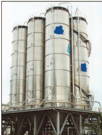
Weight limit is unlimited, although the number of vessel supports typically should not exceed eight.
