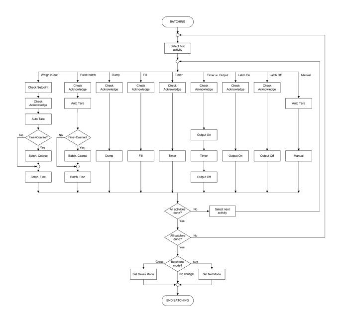
Principles how batching is carried out. The batching sequence can include up to twelve activities.
