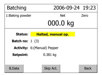
Alternatively the instrument can be set to allow manual entry of the added material weight value.
