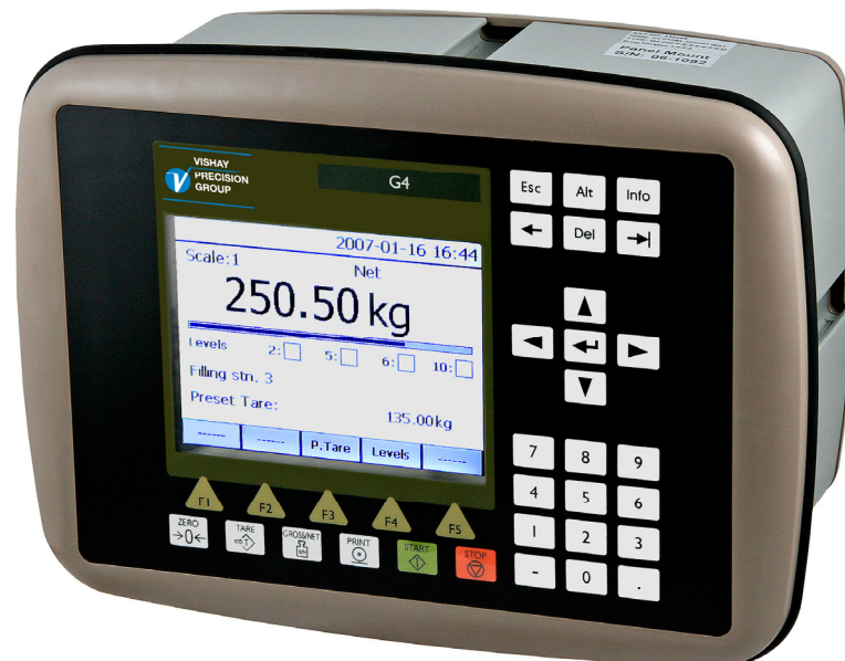
Front panel of the G4 instrument with color touch display, five function keys below the display, six application specific keys, numerical keypad, joystick keypad (arrow keys), Esc, Alt, Backspace, Delete, Tab and ENTER keys. In addition there is an Info key that is used to access the instruments menu system.
