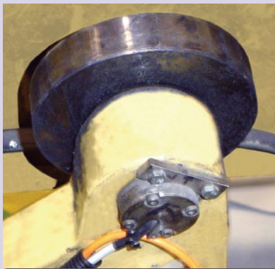
Secondary arm load cell is mounted directly onto the spool reel
