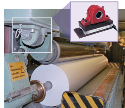
Load cells mounted under rider roll
