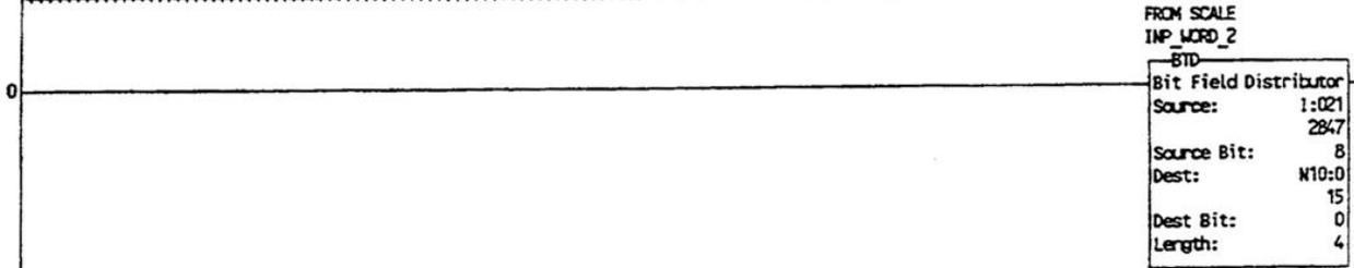
+SHIFT STATUS ID BITS FROM INPUT WORD 2 (BITS 12-15 DECIMAL or 14-17 OCTAL) TO GENERATE THE STATUS ID CODE (00-15):
