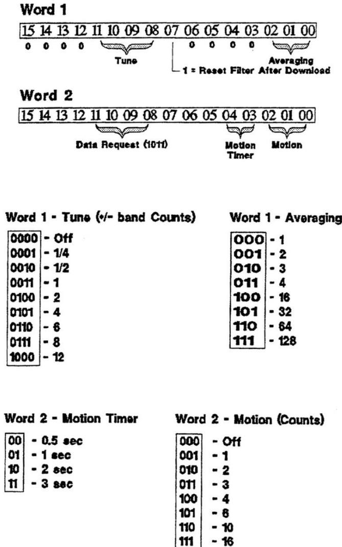
**Figure 2-5. Filter Data Bits Selections**
