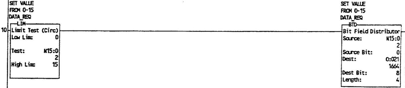
NO DOWNLOAD: IF A VALUE IS PLACED IN N15:1 AND USER PUSHBUTTON "NO\_DNLDR" IS DEPRESSED. THE VALUE IN N15:1 WILL BE PUT IN THE APPROPRIATE BITS OF SCALE OUTPUT WORD 2 FOR THE COMMAND. VALID VALUES AND FUNCTIONS ARE:
