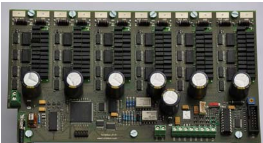
Fig. 1: Each channel uses 96 pieces of Vishay Foil Resistors' VSRJ 0.01% Bulk Metal Foil resistors
