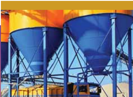
Load cells and weighing systems transform standard silos into scales for inventory or true weight detection
