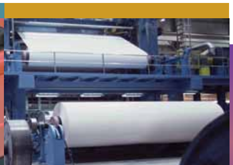
Reel Optimizing System measures and optimizes web tension to minimize wrinkles in paper and reduce scrap
