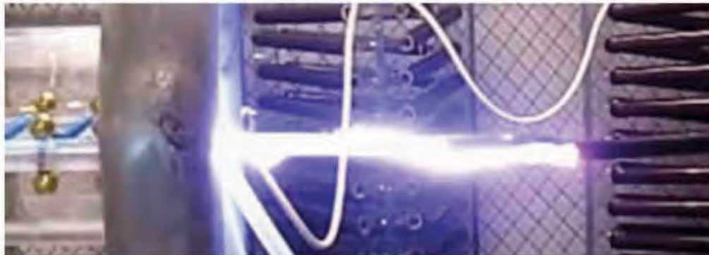
Figure 10. CUT#5. Photo of flashover. Positive polarity.
