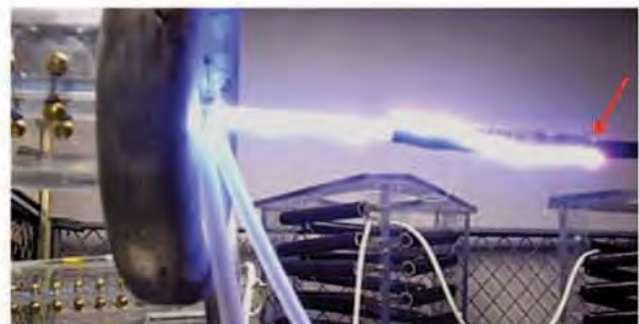
Figure 11. CUT#6. Photo of flashover. Positive polarity.
