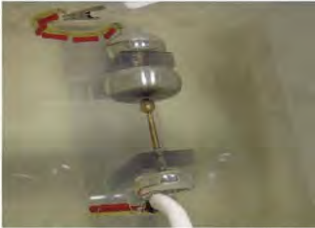
Figure 6. Limiting resistors (in red) attached to the electrodes. Note the soot floating in the oil.
