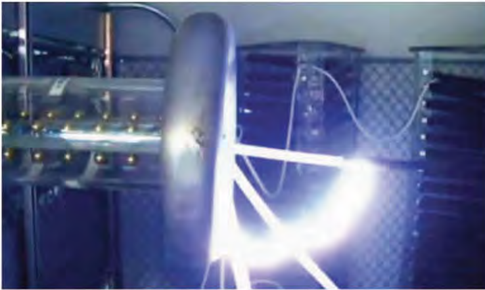
Figure 9. CUT#4. Photo of flashover. Positive polarity.
