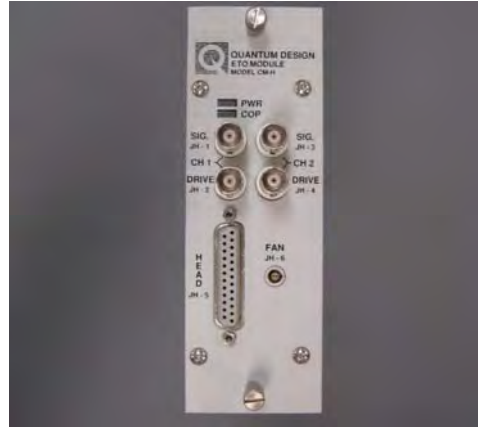
Figure 3-2. Picture of the ETO module front panel showing the CH1 1 measured signal BNC (JH-1), CH1 drive signal BNC (JH-2), CH2 measured signal BNC (JH-3), CH2 drive signal BNC (JH-4), the head cable connector (JH-5), and the fan cable connector (JH-6).
