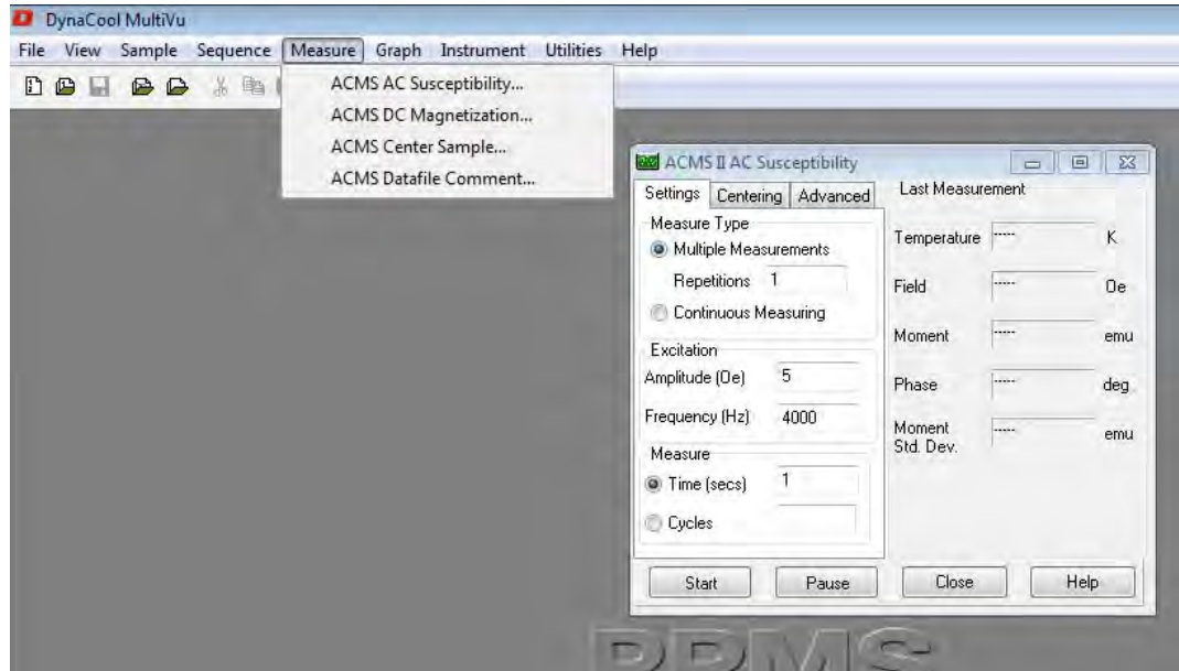
Figure 6-6. ACMS II immediate-mode commands in the context of the MultiVu window and the Measure dropdown menu
