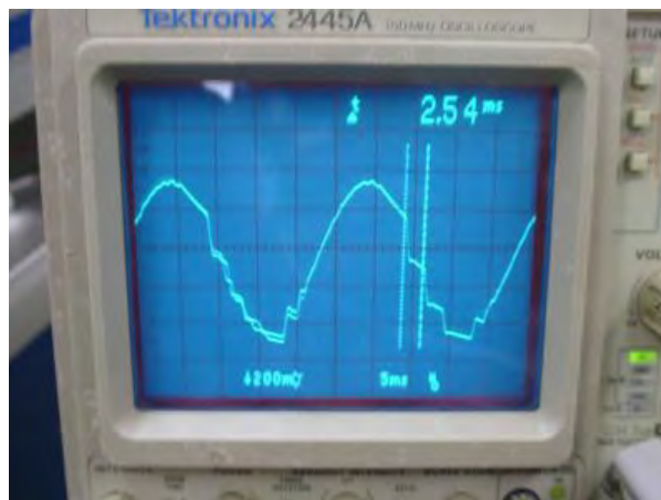
Figure 7-5. Oscilloscope trace of 40 Hz coilset signal, measured at the BNC on the VSM module. Note the jagged distortion of the signal, which would be smooth and sinusoidal for a well-mounted sample.
