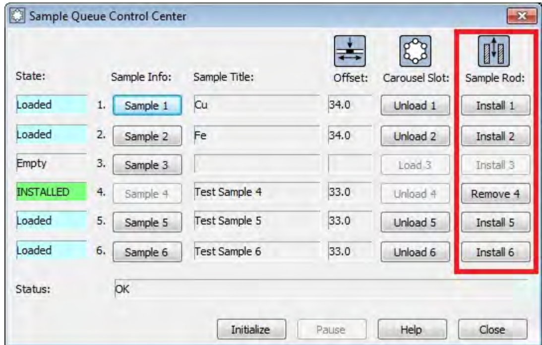
Figure 4-7. Sample Rod column in the Sample Queue Control Center.
