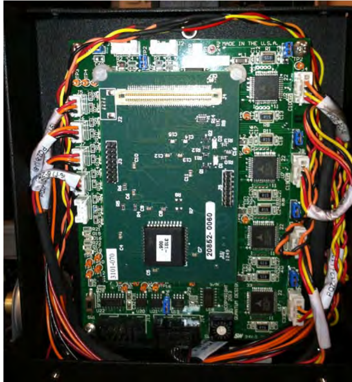
Figure 3-6. Sample Queue Control Module
