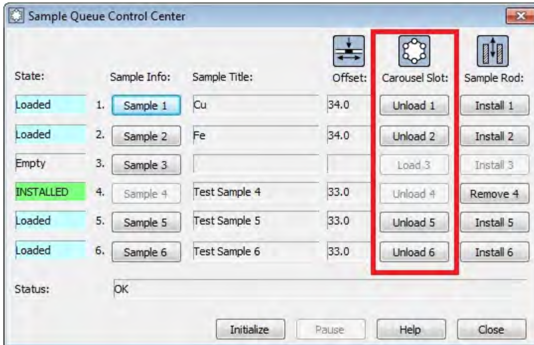
Figure 4-6. Carousel Load/unload button in the Sample Queue Control Center.
