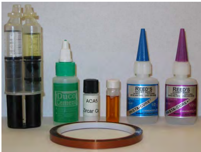
Securing agents from the left: 2-part epoxy; Duco cement; ZircarCement; GE7031 Varnish; fast curing Superglue; slower curing Superglue; Kapton tape.
