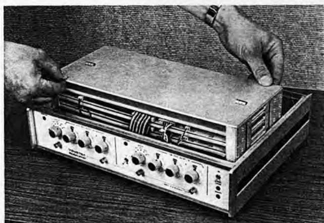
Figure 5-3. Moving Card Cage Out of Instrument
