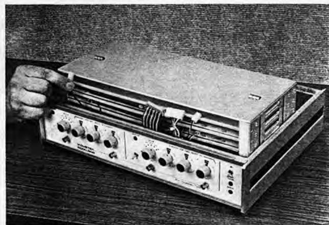
Figure 5-4. Disconnecting Board Connectors
