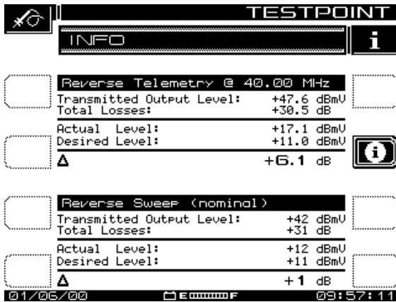
Fig. 4-4 Telemetry and Sweep Generation and Injection Levels
