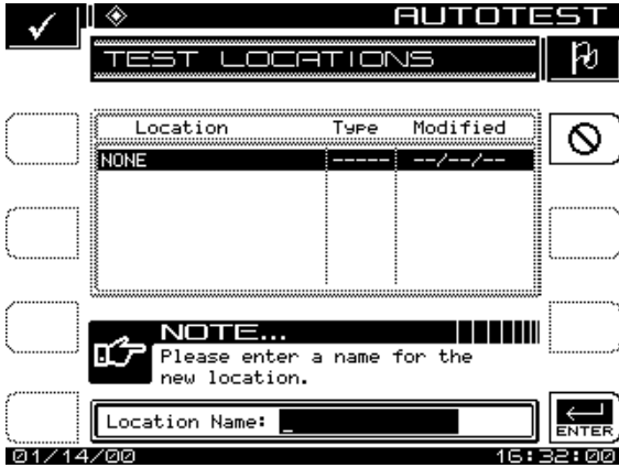
Fig. 13-25 Naming a Test Location
