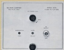
Model 6223 4.0 to 12.4 GHz: Extends coverage to the C and X bands. When coupled with the Model 6215, coverage is extended from 1 to 12.4 GHz.
