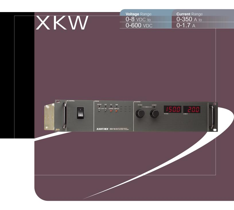
Xantrex's XKW Series is a proven product, available in nineteen 1000 watt and 3000 watt models. High frequency conventional PWM switching is used to achieve high power density in compact 19-inch rack packages 1.75 inches (1 U) high for the 1000 watt model and 3.5 inches (2 U) high for the 3000 watt models.
