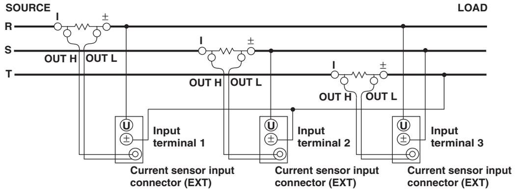
**Wiring Example of a Three-Phase, Four-Wire System (3P4W) Using a Shunt-Type Current Sensor**
