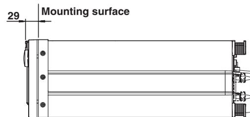
Unless otherwise specified, tolerance is  $\pm 3\%$  (however, tolerance is  $\pm 0.3$  mm when below 10 mm).
