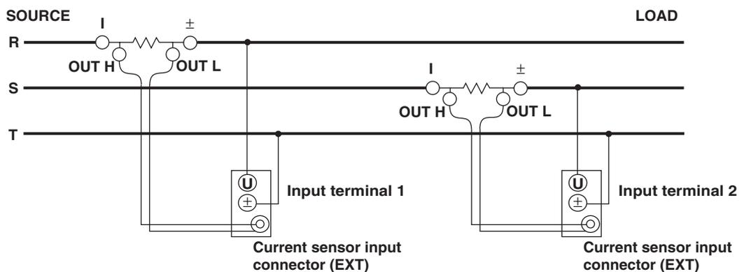
**Wiring Example of a Three-Voltage, Three-Current System (3V3A) Using a Shunt-Type Current Sensor**
