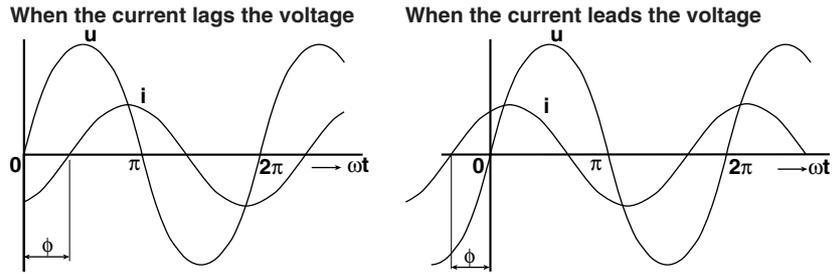
The vector display is used to show the amplitude and phase relationships of the voltage and current. Taking the positive vertical axis to be the reference, an angle in the counter clockwise direction is taken to be positive.
