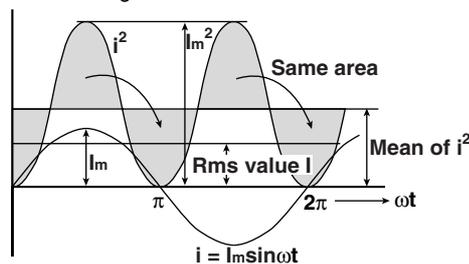
The rms value (effective value) is the value of the DC signal that generates the same heating effect as the AC signal. If the value of the DC signal that generates the same heating effect is expressed as  $I$ , then
