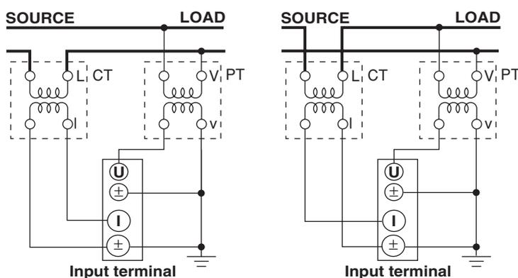
**Wiring Example of a Single-Phase, Three-Wire System (1P3W) Using PT and CT**
