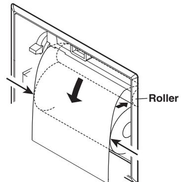
Align the left and right edges of the paper as it exits the printer so that they are even with the sides of the roll.
