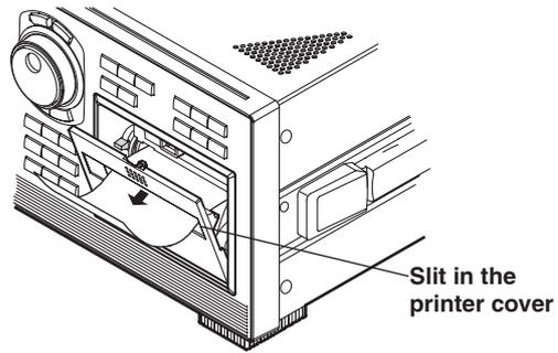
10. Close the **printer cover**. Firmly press the section marked as PUSH until it clicks in place.
