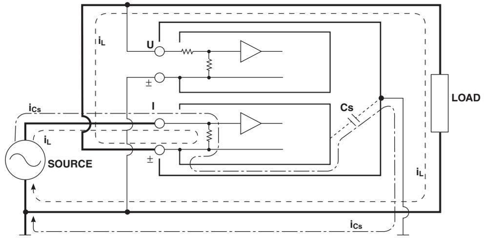
When measuring high frequencies as in this instrument, this error,  $i_{Cs}$ , cannot be ignored. By connecting the current input terminal of the instrument to the side that is close to the earth potential of the power source (SOURCE), the terminal of the current measurement circuit of the instrument approaches the earth potential. Thus,  $V_{Cs}$  becomes approximately zero and very little  $i_{Cs}$  flows.
