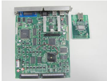
DL with the Ether Board Assy Removed
