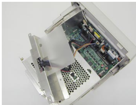
DL with the I/O Device Removed
