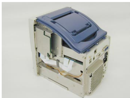
DL with the Top Cover Removed
