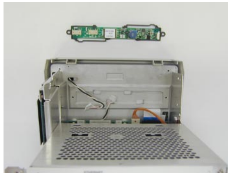
DL with the Inverter Assy Removed
