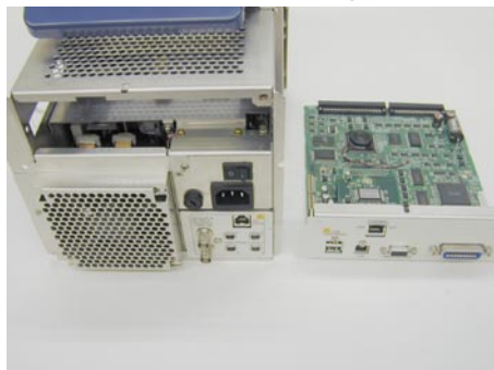
DL with the CPU Board Assy Removed
