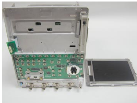
DL with the LCD Removed
