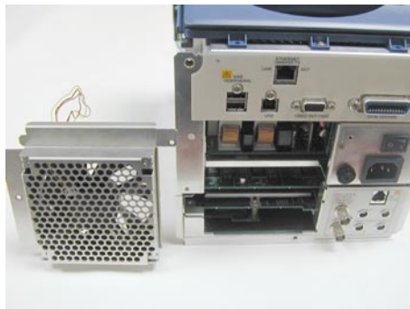
DL with the Fan Assy Removed
