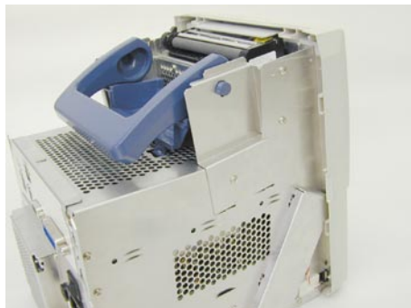
DL with the Printer Case Removed
