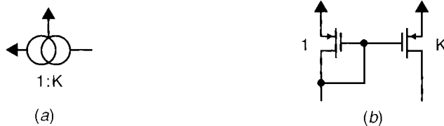
Fig. 6.8 (a) A symbol representing a current mirror. (b) Example of a simple current mirror.
