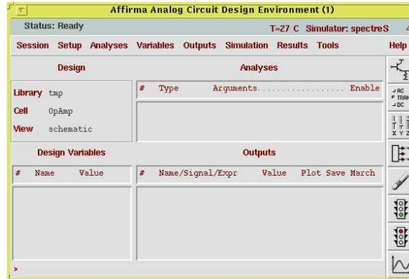
Figure 1.7: *Affirma Analog Environment Simulation Window*
