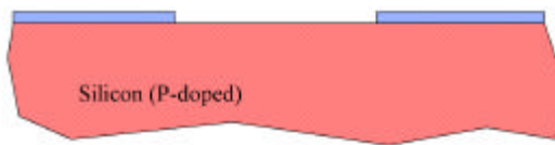
Fig. 1-6: The oxide is etched away and the photoresist is removed.
