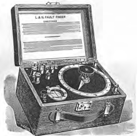
2-18 'Fault-Finder' Bridge L&N Before 1912
