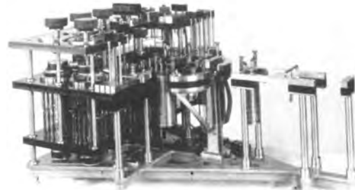
2.20 NBS High-Precision Bridge or 'Wenner Bridge' Removed from Oil Bath 1940
