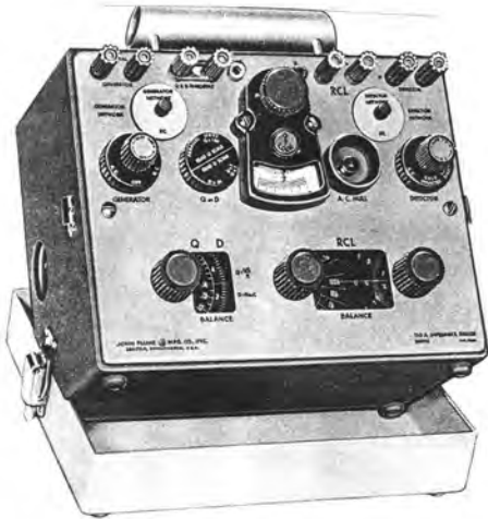
3-7 Impedance Bridge Fluke Type 710A 1962
