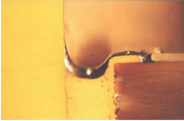
Figure 9-29: Microsection showing a satisfactory solder joint after reflow of the through-hole pin.
