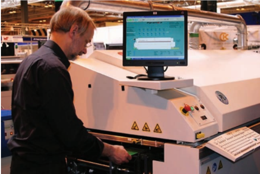
Figure 5-3: BTU Convection reflow system used on the SMART Group Lead-Free Experience technology feature and typical of the systems used in medium- and high-volume production.
