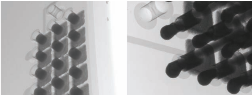
Figure 3-7: X-ray photographs show the degree of fill before (left) and after (right) lead insertion. X-ray used before through-hole assembly to assess the volume of solder paste fill after printing is recommended to check for paste voids or measure the variation in the printing process.
