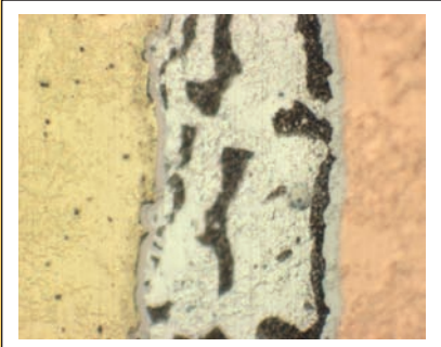
Figure 8-8: SnPb solder on Cu PCB finish
