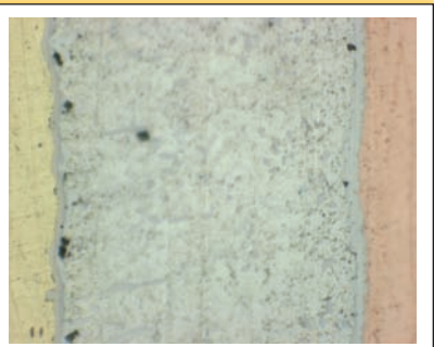
Figure 8-7: SnAgBiCu solder on tin PCB finish
