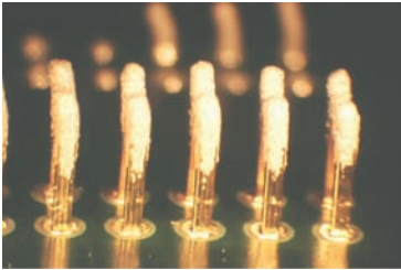
Figure 9-21: Excessive paste push-out.
