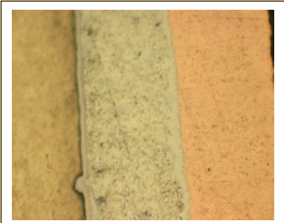
Figure 8-4: SnAgCu solder on Cu PCB finish
