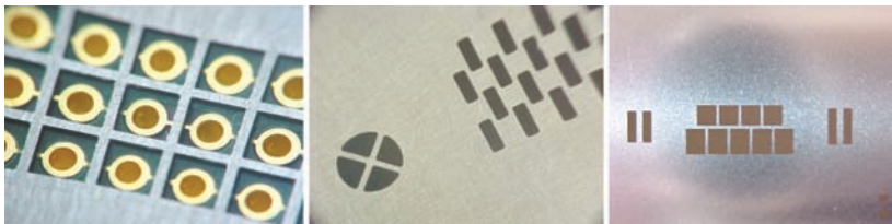
Figure 3-17: Examples of different stencil apertures aligned with the printed board prior to printing.
