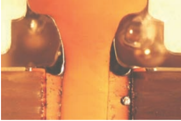
Figure 9-23: Microsection of a pin grid array lead showing a satisfactory solder joint at the base of the pin.
