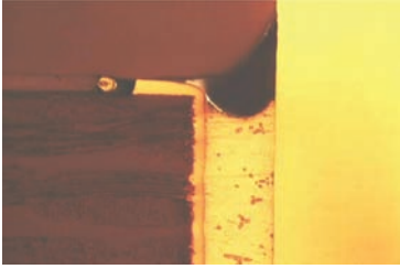
Figure 9-27: Solder ball visible on the surface of the board after micro-sectioning.
