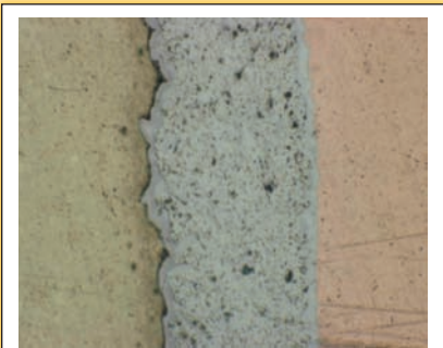
Figure 8-6: SnAgBiCu solder on tin/lead HASL
