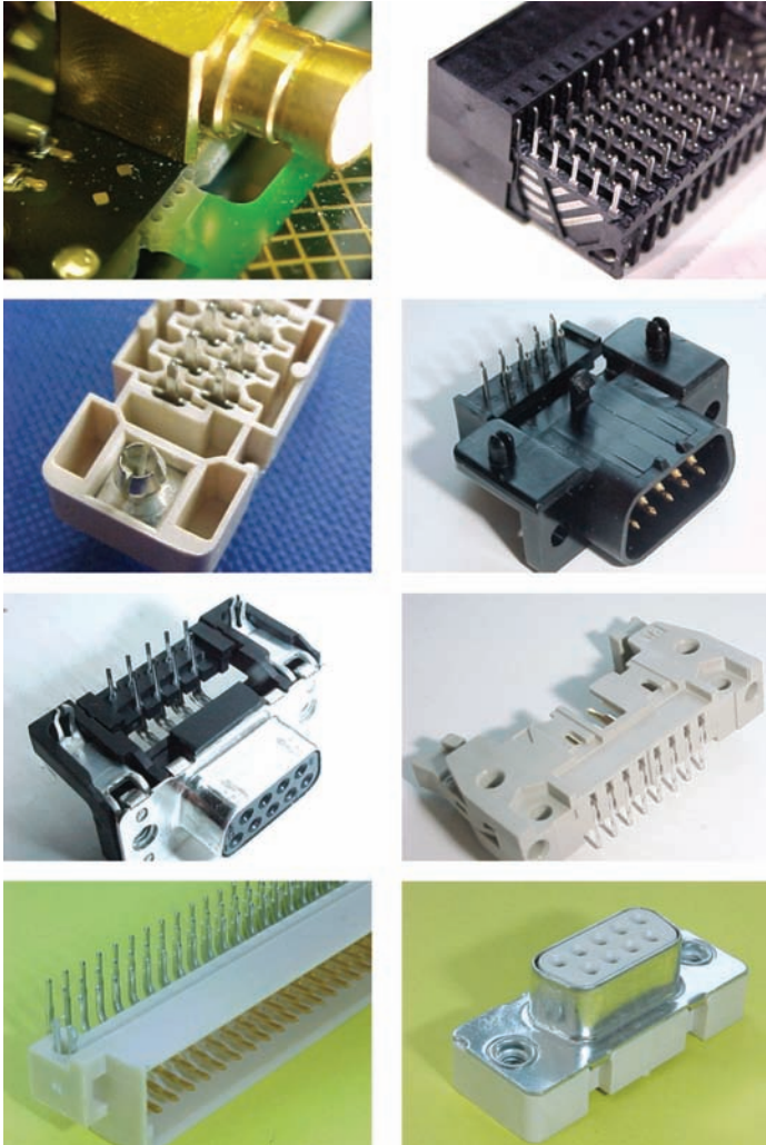
Figure I-5: Samples of different components that could be assembled using PIHR.
