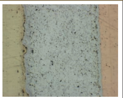
Figure 8-5: SnAgBiCu solder on Cu PCB finish
