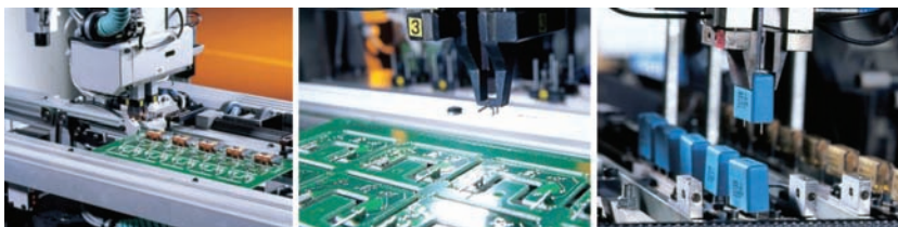
Figure 4-4: Close-up view of component insertion with odd form insertion systems supplied by PMJ.
