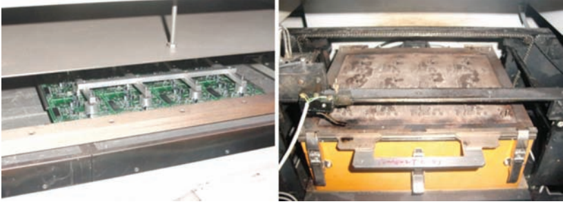
Figure 3-12: (Left) Hold down/support fixture being used on through-hole components to hold the board rigid. (right) Reflow step where hot air is blown directly onto the through-hole lead and paste deposits to allow reflow.
