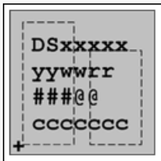
Figure 4. Top marking for the SFN package. This is topside view and contacts are not visible.
