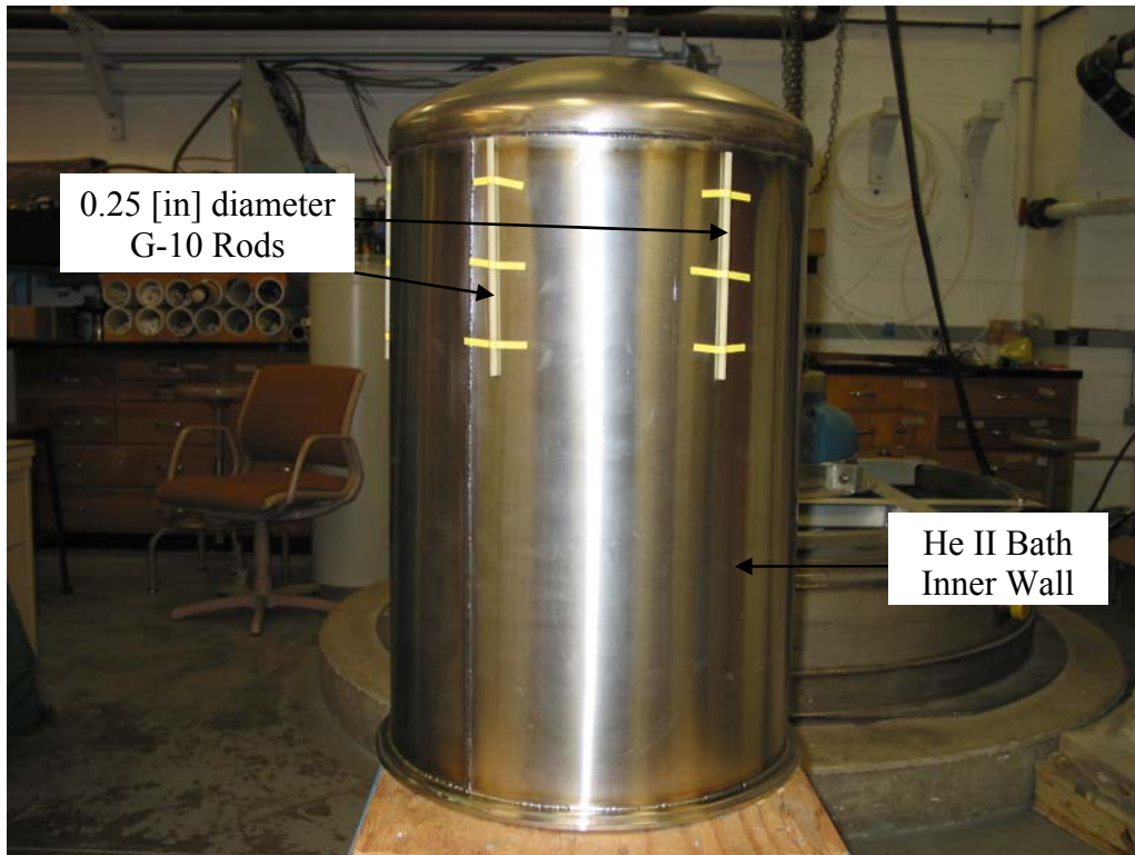
Figure 2.16. The He II bath inner wall with G-10 rods taped to it in order to avoid direct contact with the outer wall.
