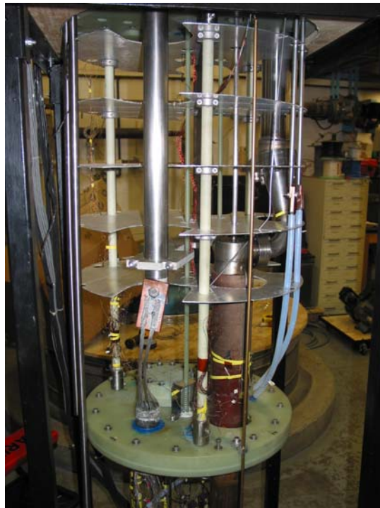
Figure 2.30. Radiation shields installed on the cryostat.
