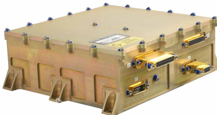
Figure 16. NGAS HEC dual-piston, linear-motor pulse tube cooler drive electronics [Harvey, et al., 2004].
