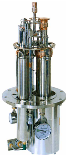
Figure 23. Sumitomo hybrid Gifford-McMahon/JT coldhead for 4K cooling.
