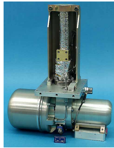
Figure 15. NGAS dual-piston, linear-motor HEC pulse tube cooler [Raab and Tward, 2010].
