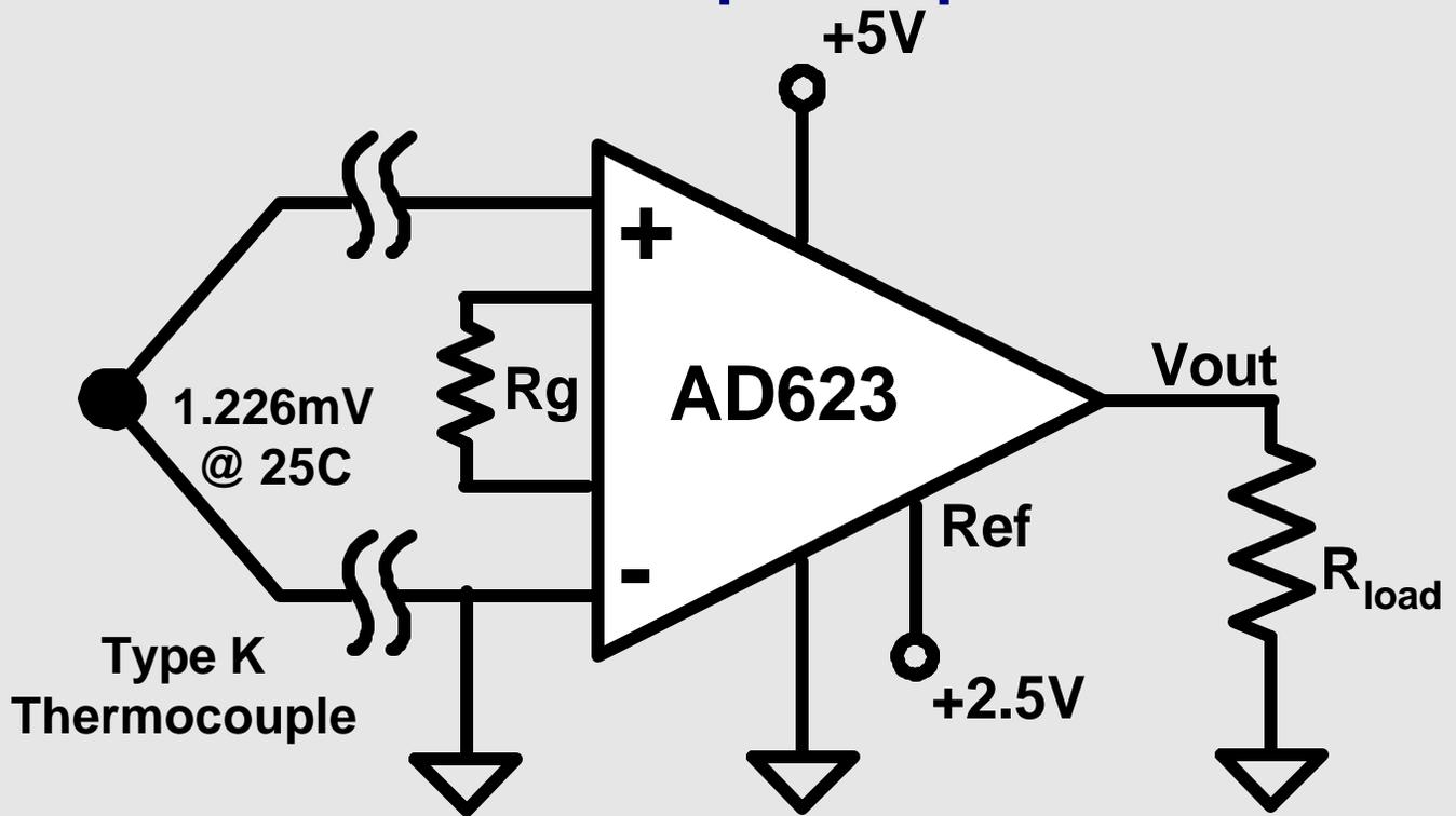
**Useable common-mode voltage range extends to 0V even with a single supply.**
