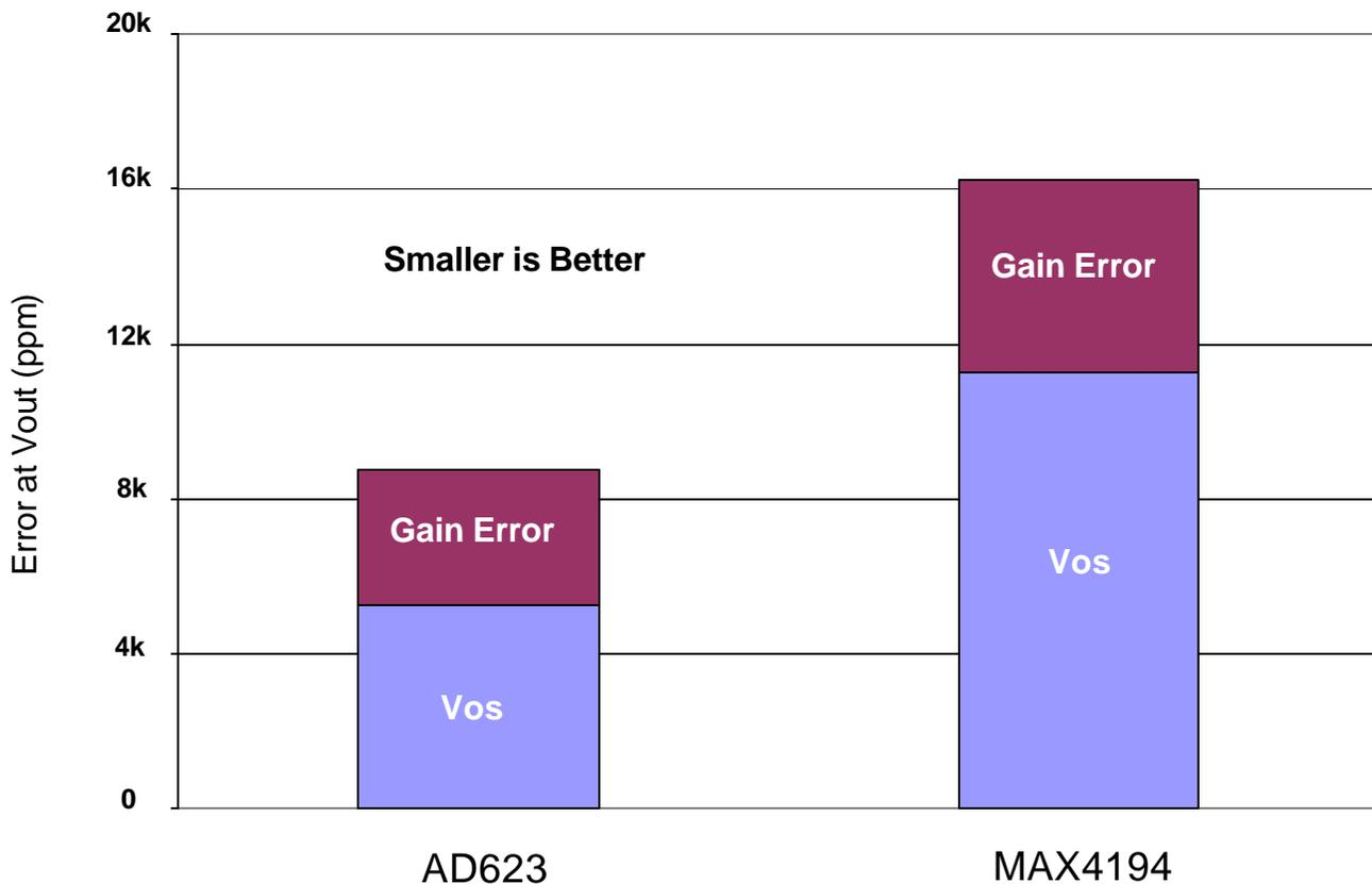
**The AD623 is an excellent thermocouple amplifier.**
