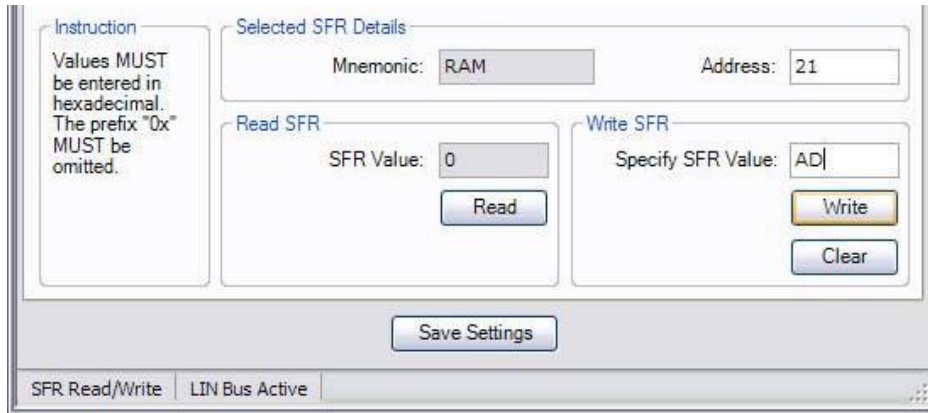
Fig. 9 – Read/Write RAM (e.g. write 0xAD to RAM location 0x21)
