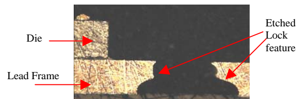
Fig.4. Leadframe locking features
