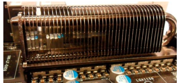
Example: Motherboard (PCB 4 layer, 35 μm) with high performance heatsink
