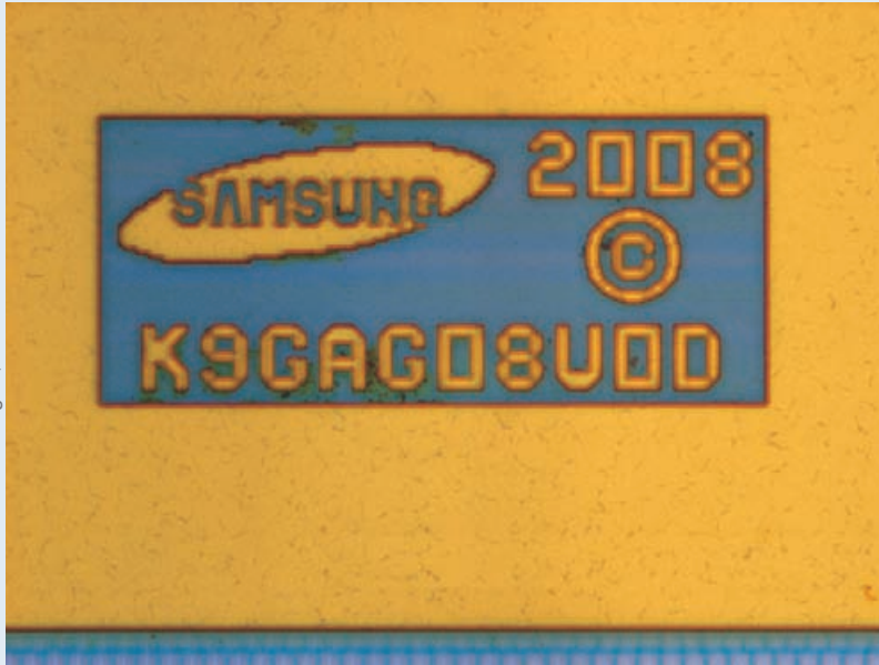
Die Markings of the Samsung 42nm 16 Gbit NAND Flash
