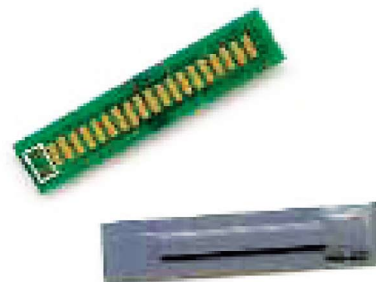
Figure 1. AT77C104B FingerChip IC.
