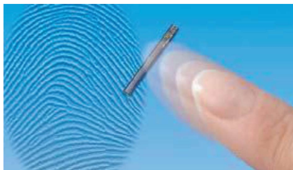
Figure 2. Typical fingerprint—and finger being swept over a sensor.
