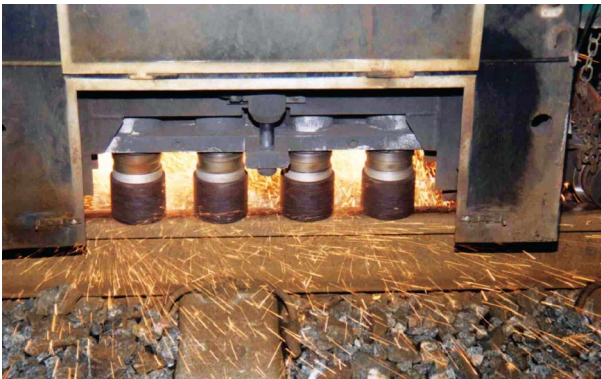
Figure 11. Electronic maintenance plans are deployed to maintenance machines, which solve the problem on-rail by grinding.
