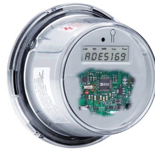
Figure 2. Solid-state electronic energy meter.
