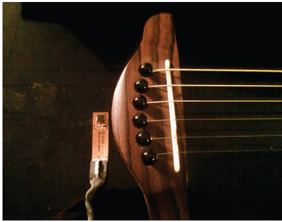
Figure 7. Accelerometer mounted on Fender Stratocoustic acoustic guitar.
