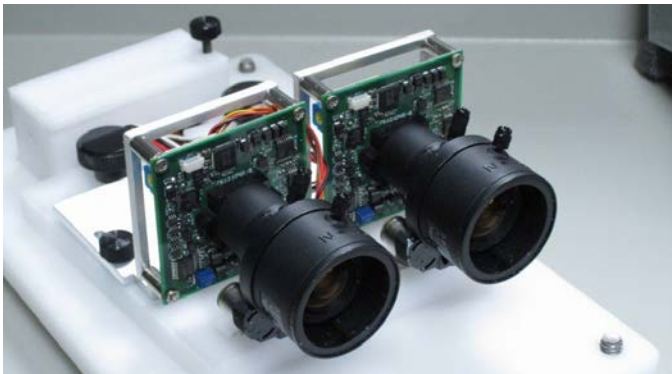
Figure 1. Two cameras on a stand aligned for stereoscopic vision.
