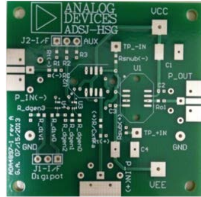
Figure 6. Evaluation board for amplifier including digital potentiometer connection.
