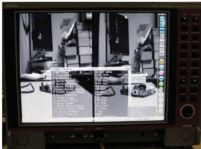
Figure 15. Side-by-side 576p picture with video timings
