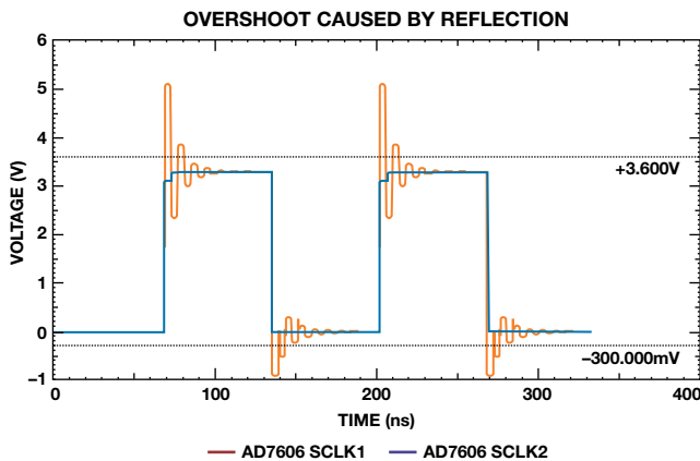
Figure 8. AD7606 IBIS model simulation of overshoot.
