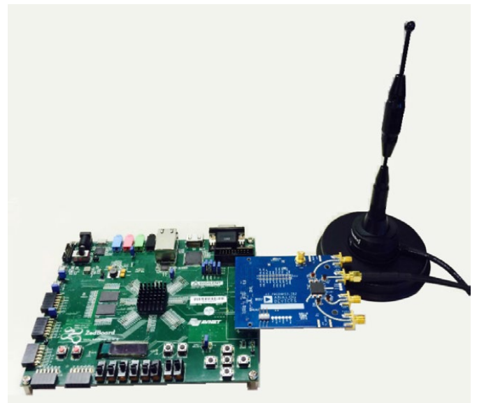
Figure 2. Hardware setup for ADS-B algorithm validation.
