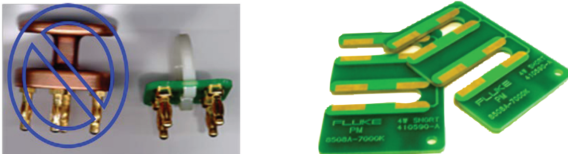
Figure 1. Small shunting devices are shown here. Specially made circuit boards, supplied with Fluke's 8508A DMM, provide both ohmic and thermal zeros for quick stabilization.
