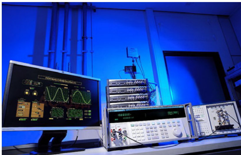
A commercial high-precision calibrator (center) is calibrated by means of the AC quantum voltmeter in the AC voltage mode.
