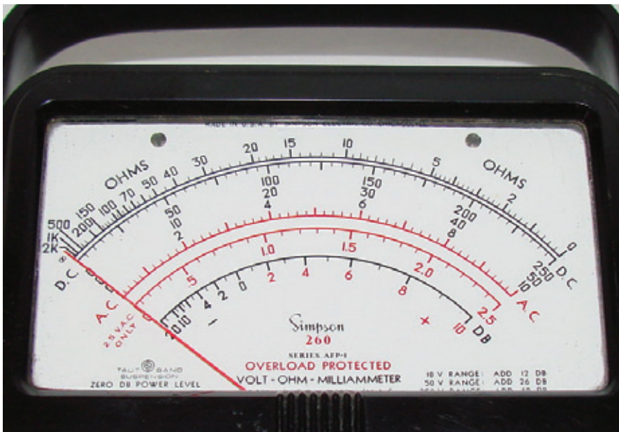
Figure 1. Meter face of the Simpson 260. Picture courtesy of simpson260.com.
