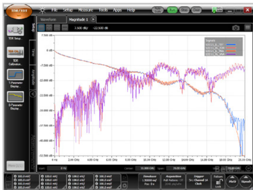
Figure 11. Insertion Loss, SDD21, and Return Loss, SDD11, measured using TDR and VNA.
