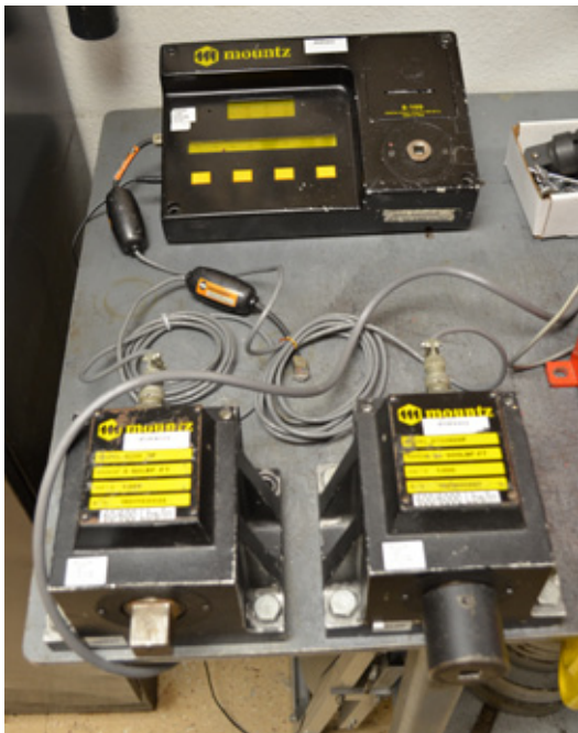
Figure 1. Typical torque calibration system.
