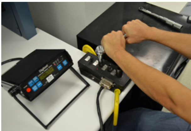
Figure 2. Exercising the transducer.
