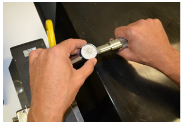
Figure 3. Leveling the torque wrench.
