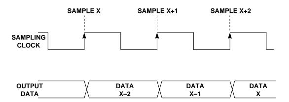
ABOVE SHOWS TWO CLOCK-CYCLES PIPELINE DELAY
