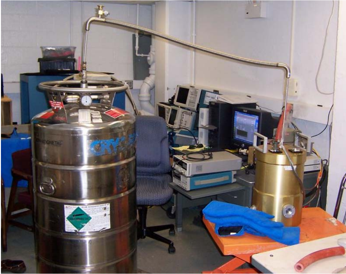
Figure 11: Helium transfer from storage Dewar to test Dewar
