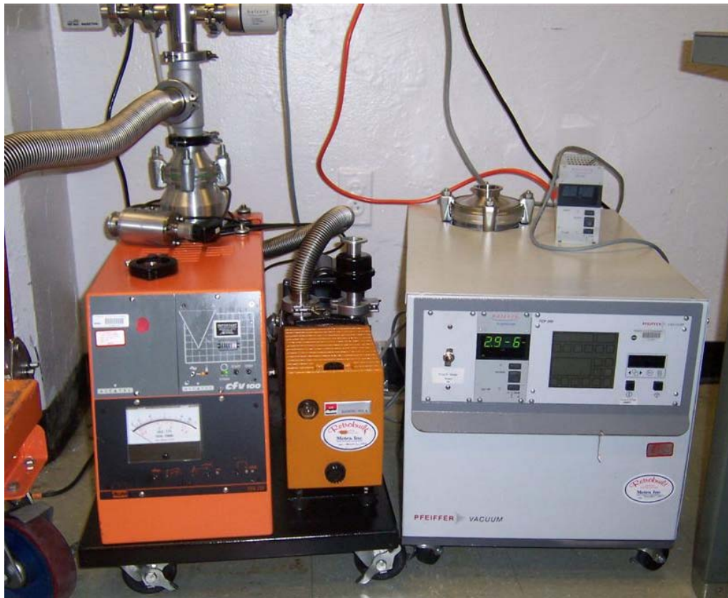
Figure 8: Alcatel pump and controller (left) and Balzers pressure gauge (right)
