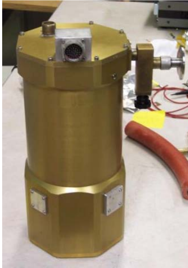
Figure 5: Infrared Laboratories Test Dewar used for this research
