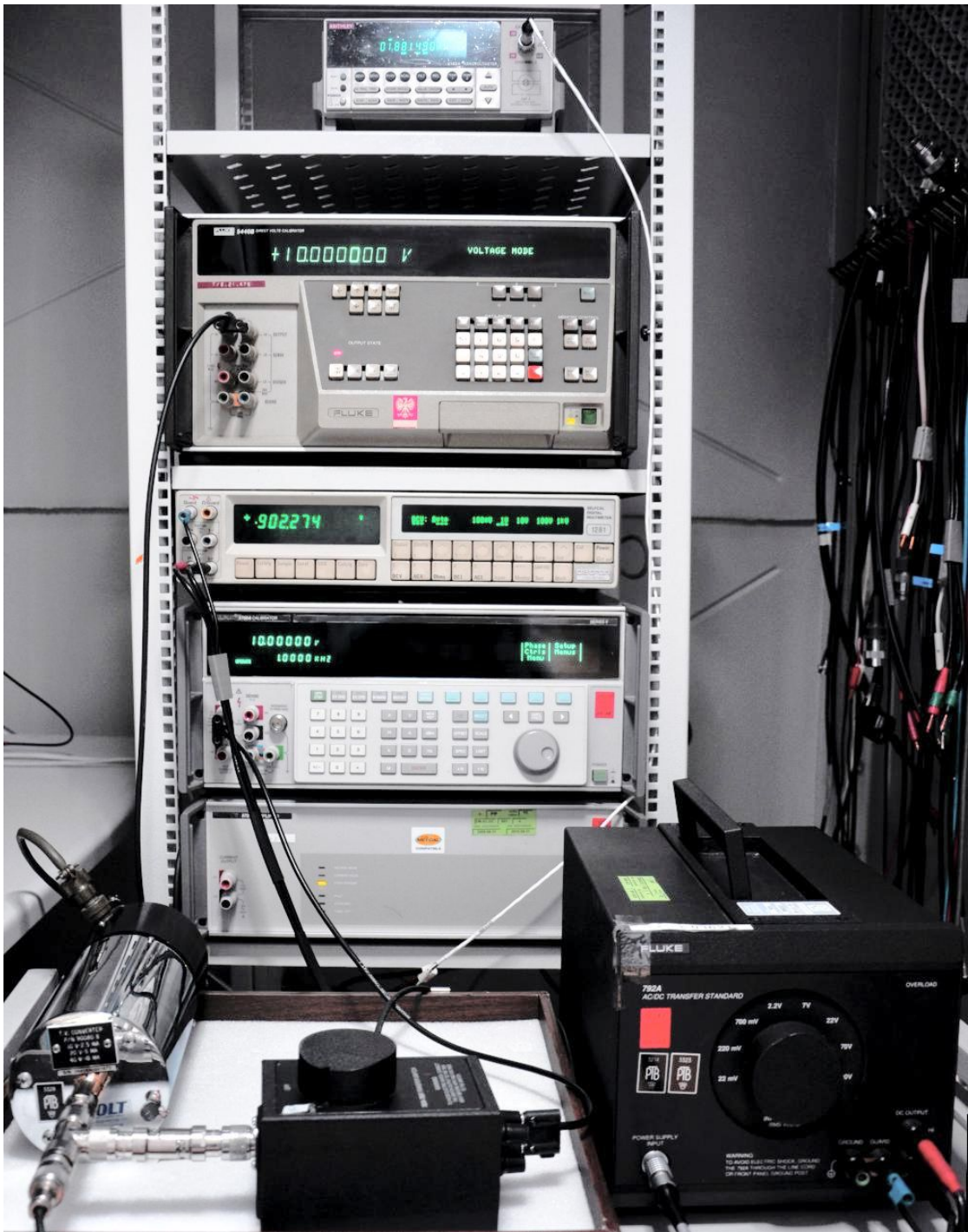
Figure 11.6: AC-DC difference comparator system placed in GUM. The measuring station consists: DC voltage sources FLUKE 5440B calibrator, AC voltage sources FLUKE 5720A/5700A calibrator, Keithley 2182A nanovoltmeter, AC-DC Voltage Tee, reference converter HOLT model 11, UUT Fluke 792A.
