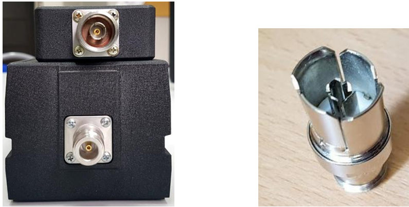
Figure 11.7: Left: male (upper) and female (lower) N connector. Right: GR874 hermaphroditic connector.
