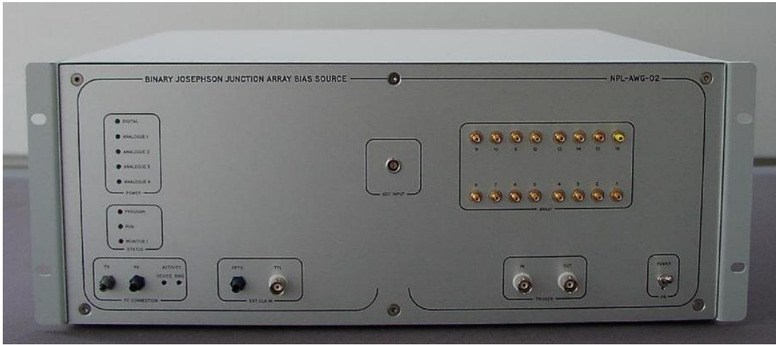
Figure 2.5: NPL Josephson array bias source.
