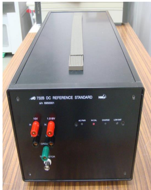
Fig. 1: An upgrade-box with Fluke 732B and additional batteries
