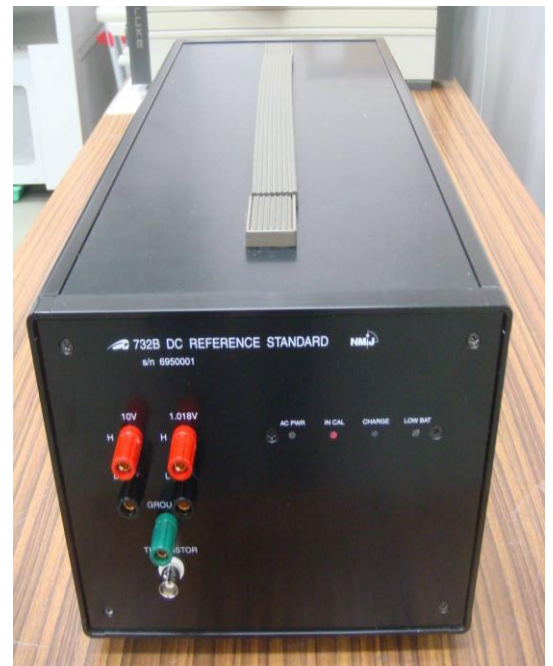
Figure 4-1 An upgrade-box for Fluke 732B with additional batteries inside.
