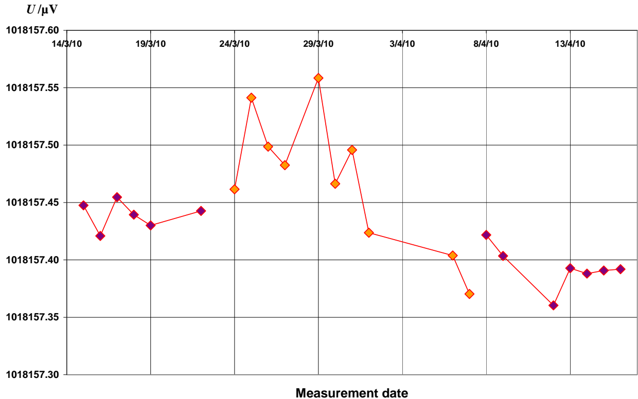
Figure 4. Voltage evolution of the simple mean of the two standards at 1.018 V.
