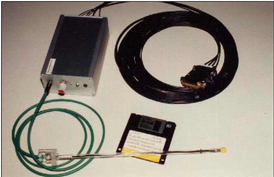
Figure 1 Electronic box with field probe and optical interface.
