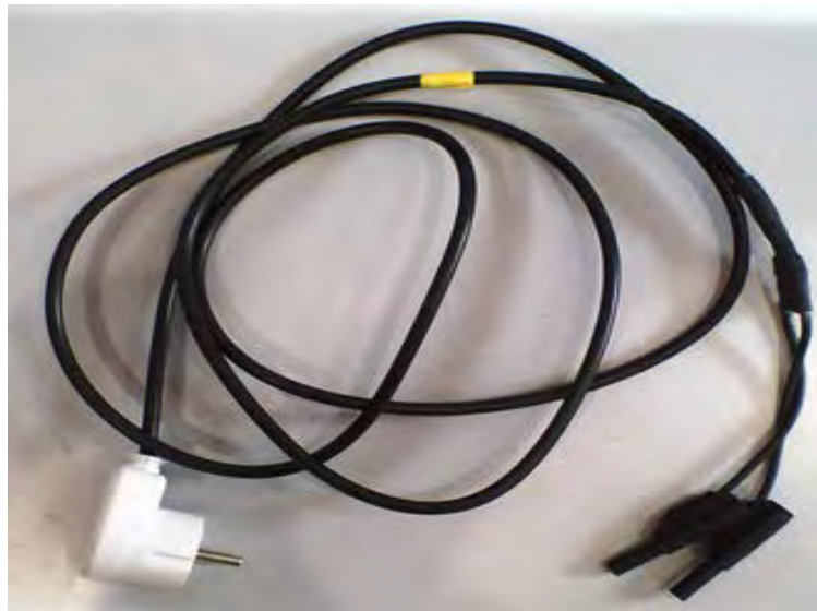
Figure 3 Power cable of travelling standard RD-33-332
