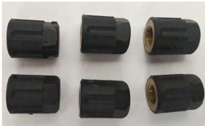
Figure 7 Clamping nuts for connection current cables of travelling standard RD-33-332
