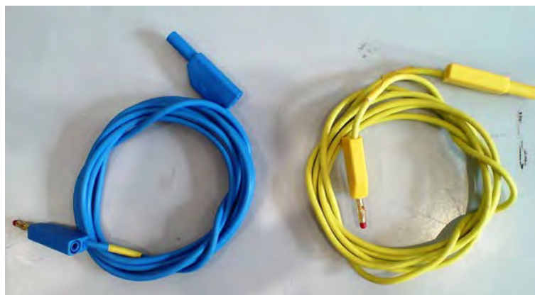
Figure 5 Voltage cables for connection travelling standard RD-33-332
