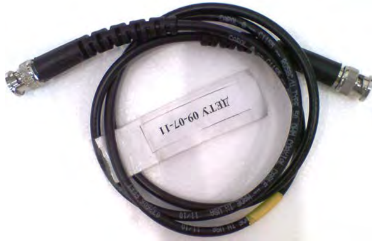
Figure 6 Pulse cable for connection travelling standard RD-33-332
