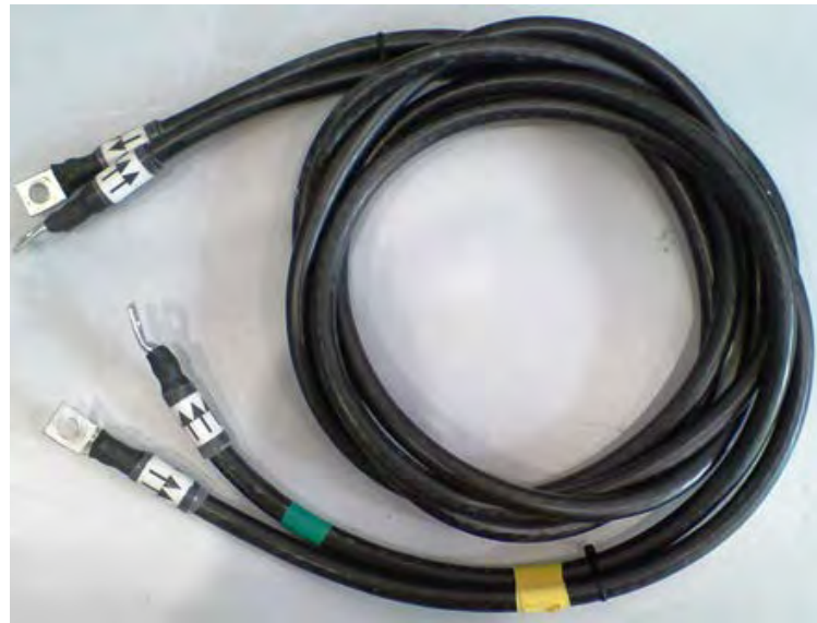
Figure 4 Current cables for connection travelling standard RD-33-332
